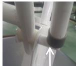
Illustration A 300kgs load applied to (spread over) both aluminium arms. No deformation evident.
