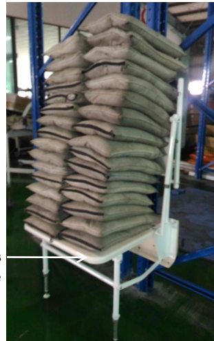
Illustration B 350kgs applied to the seat base.
