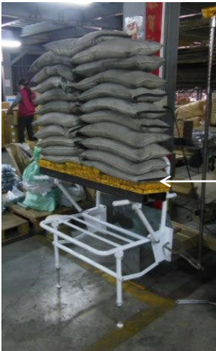
Illustration A 300kgs load applied to (spread over) both aluminium arms. No deformation evident.
